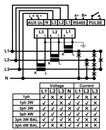
Unused Voltage terminals are internally connected Secondary of CTs must be connected to earth
